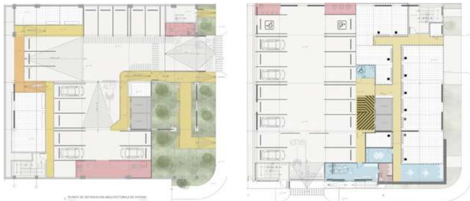
Basement and first floor layout. The blue area is the manager's office, the red area is the services, the orange area is the unloading area, and in yellow, is the pedestrian circulation. The building setback was filled with landscaping shown in green.
